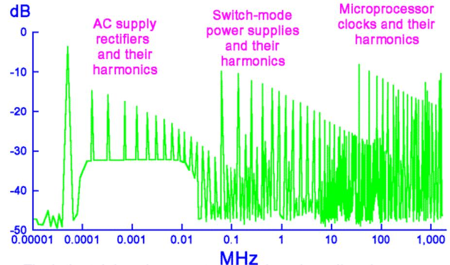
The industrial environment suffers from broadband electromagnetic interference from various instruments and devices in the plant.
