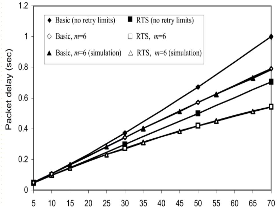
*LTE/IEEE 802.11 Latency Analysis: 10 nodes connection results in 0.1s delay. Furthermore, as the number of nodes increases the network latency largely increase.*
