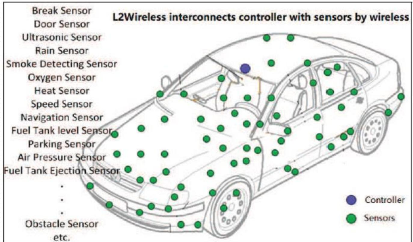
The wiring cables used for the transmission of data and power delivery within the current vehicle architecture may have up to 4 000 parts, weigh as much as 40 kg and contain up to 4 km of wiring. Eliminating these wires would additionally have the potential to improve fuel efficiency, greenhouse gas emission, and spur innovation by providing an open architecture to accommodate new systems and applications.
