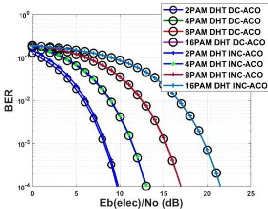
Fig. 7. BER performance of DHT INC-ACO vs DHT DC-ACO as a function  $E_{b(\text{elec})}/N_0$ .
