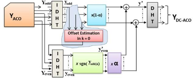
Fig. 4. Block diagram of the DHT DC-ACO.
