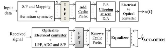
Fig. 1. Conventional ACO-OFDM block diagram.
