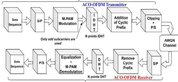
Fig. 2. Conventional ACO-OFDM block diagram.
