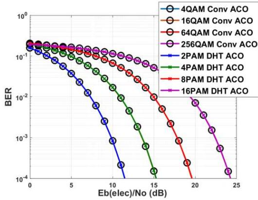
Fig. 6. BER performance of DHT ACO-OFDM vs ACO-OFDM as a function of  $E_{b(\text{elec})}/N_0$ .
